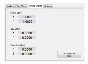
**FIGURE 15 - FIXTURE OFFSETS**
