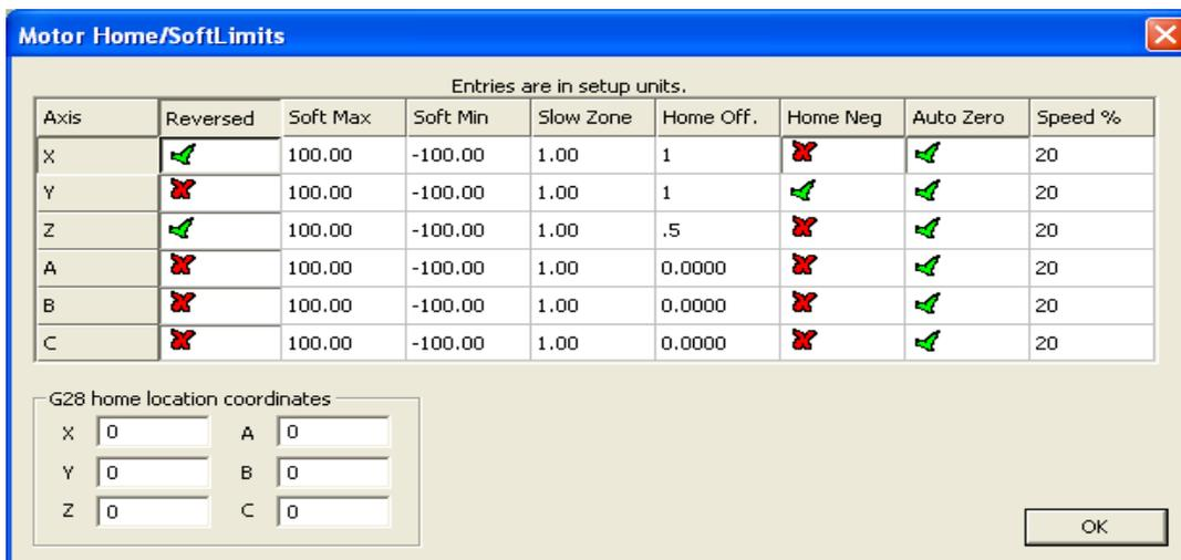
To change the axis direction, click on the Reversed column for the axis you want to change the direction. A green check mark indicates the direction is now reversed.
