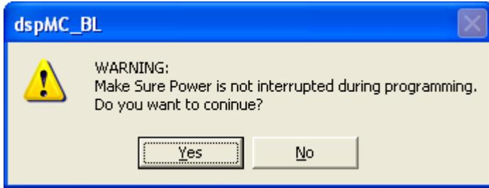
Once you click 'Yes', the software will start programming the board. The progress bar will show the programming progress. After the programming is done, the software will verify if the programming is successful. A 'SUCCESS' message is displayed if firmware programming and verification is successful as shown below.
