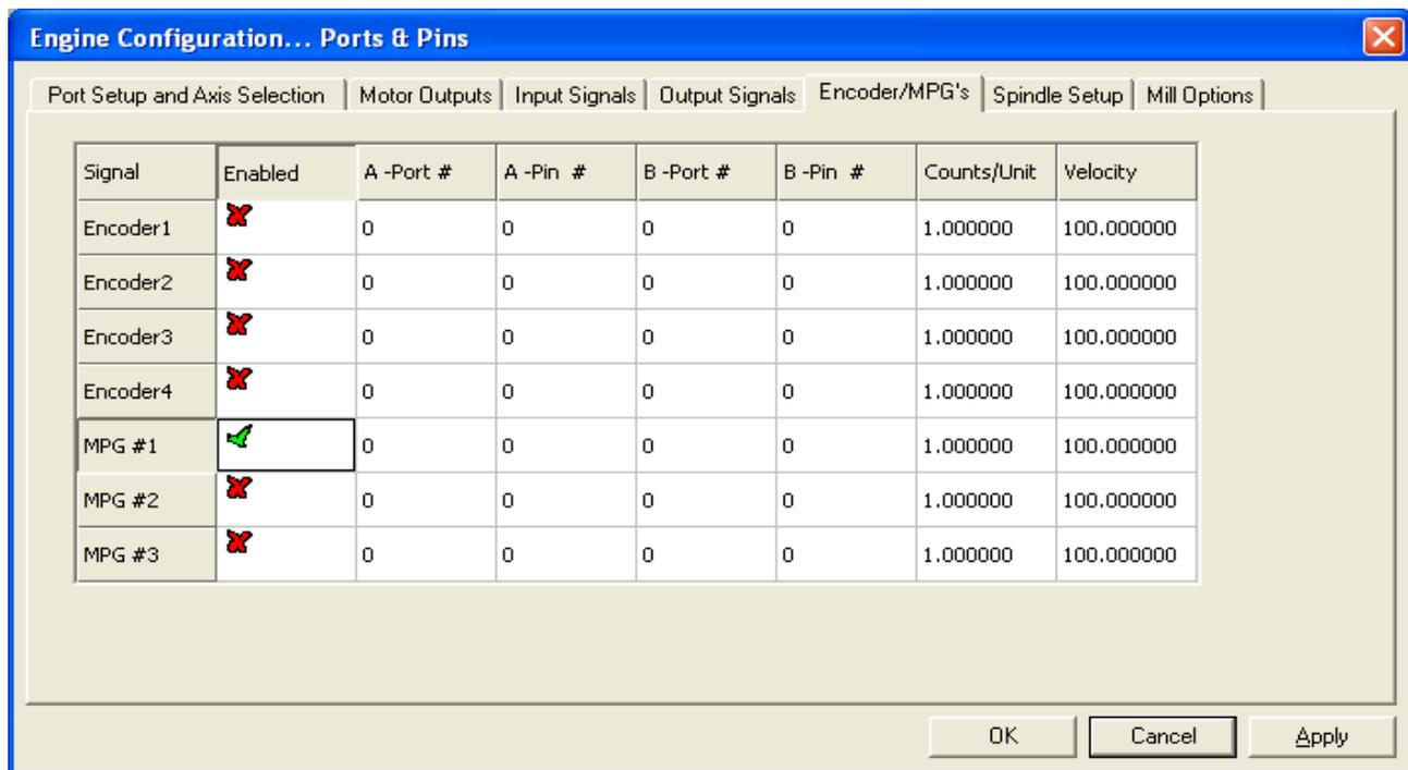
To turn on the MPG feature, make sure MPG #1 is checked green as shown above in the Ports and Pins window. The rest of the fields in this window are not used.
