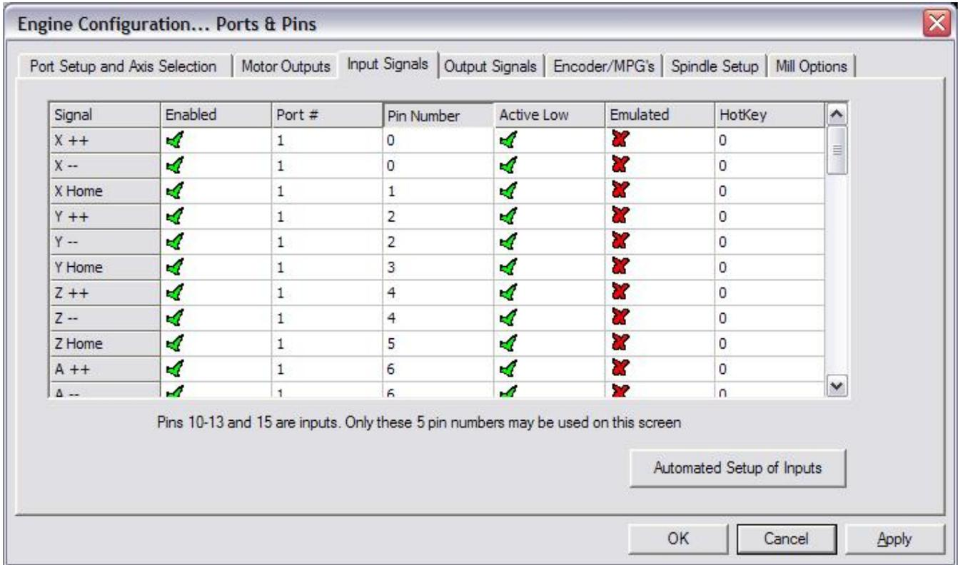
Ignore the line printed on the above window about pins 10-13 and 15. This does not apply to Interpreter 1000 based system.
