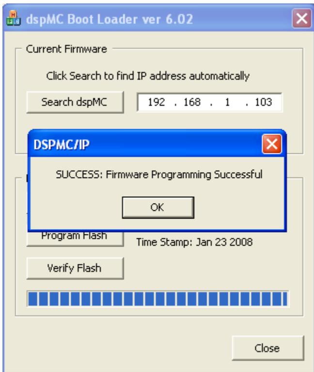
If an error is detected, it will show the location of the first data mismatch. You can try programming again by clicking on Program Flash Button to correct the error.
