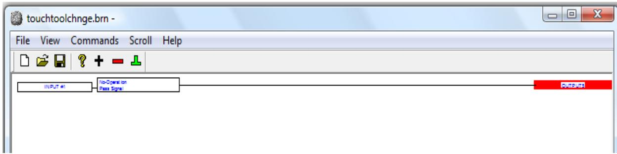
Connect a wire between input 1 and output 5 under the ports and pins tab of Mach3. After a few tries you will gain confidence and understanding.
