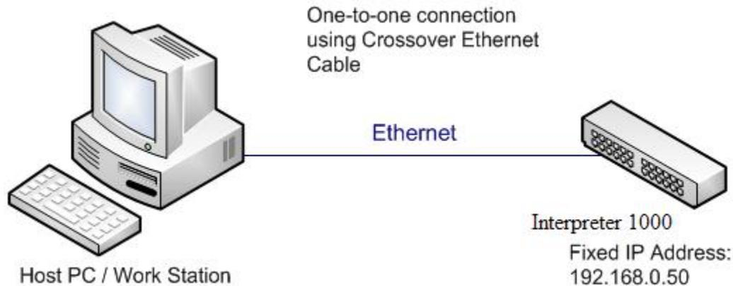
Note: If your network card has auto detection, a crossover cable may not be necessary. This setup works best when you are using the Interpreter 1000 to control a machine tool. It requires less hardware and wiring.
