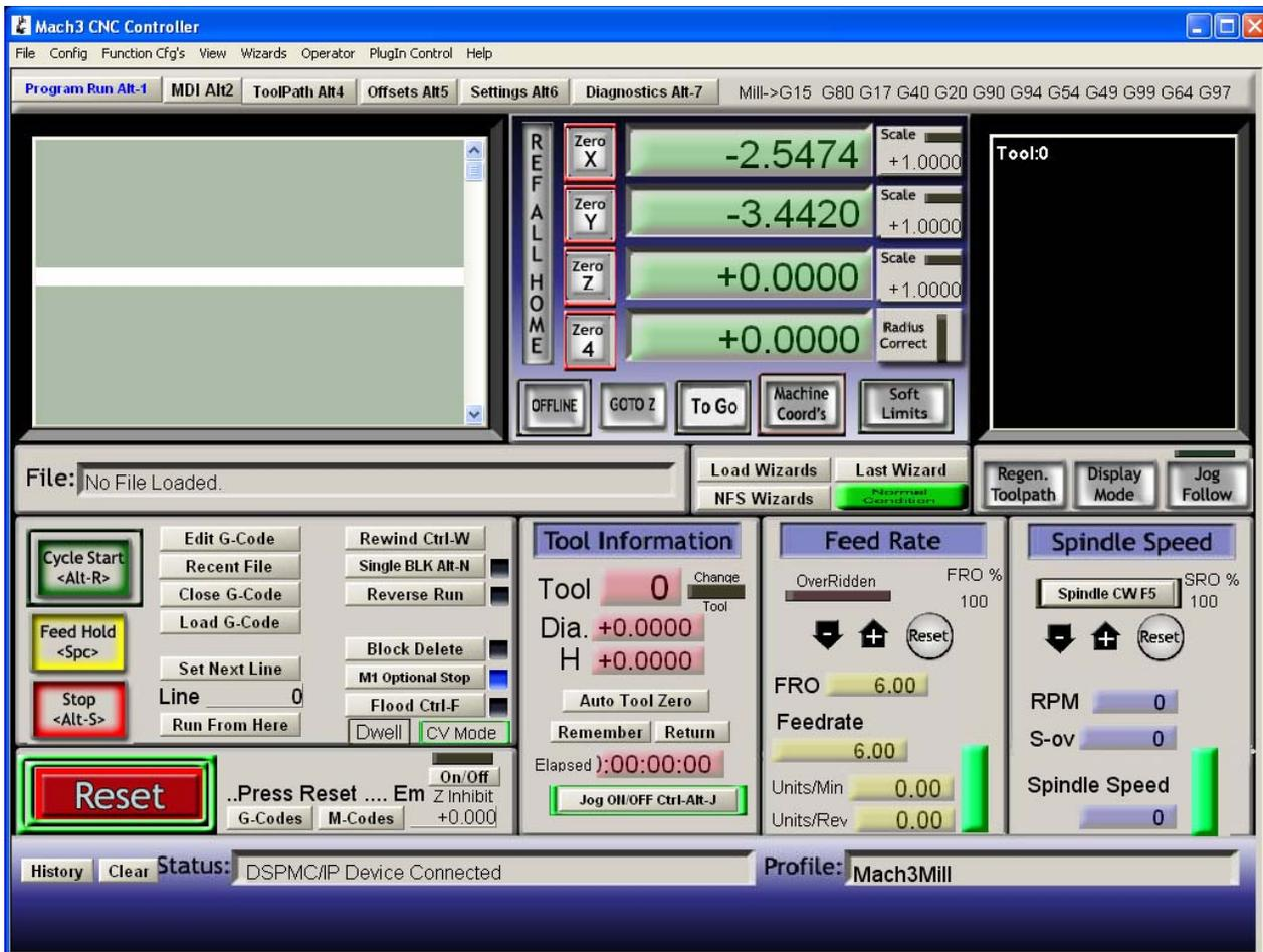
Click on the Menu item 'PlugIn Control', and then click on the item '..dspMC/IP Window' which displays the following screen indicating that the Interpreter 1000 is connected with current states of counter and other stats. User can leave this window open while running Mach3.
