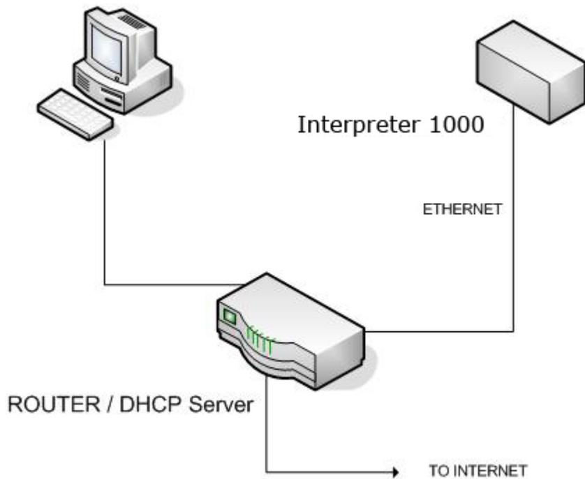
The figure above shows a basic setup using a router on your network. Connect the Ethernet cable from the Ethernet port on the Interpreter 1000 to the DHCP server/Router. Connect another Ethernet cable from the DHCP Server/Router to the PC. The DHCP server dynamically assigns IP address both to the PC as well as to the Interpreter 1000, and therefore completes the network setup without requiring any intervention from the user.
