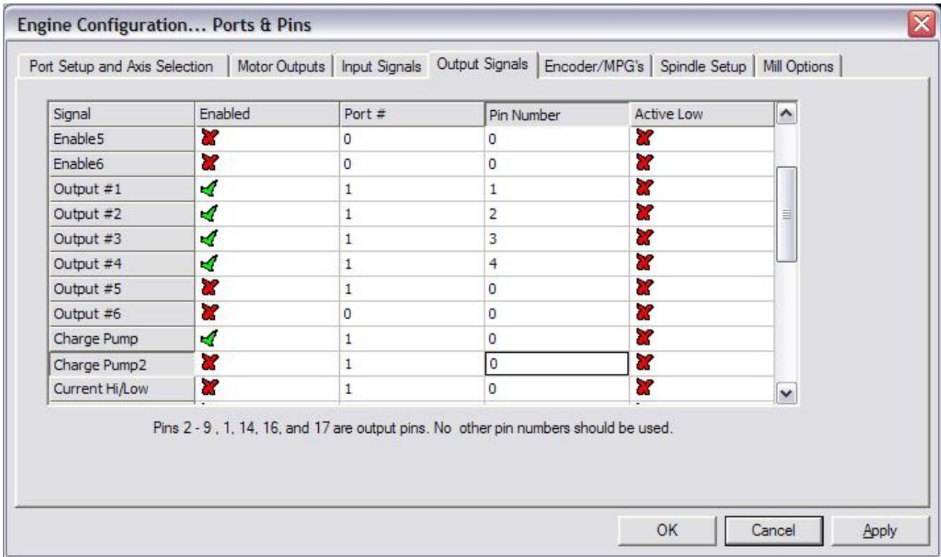
Ignore the line printed on the above window about pins 2-9,1,14.... This does not apply to Interpreter 1000 based system.
