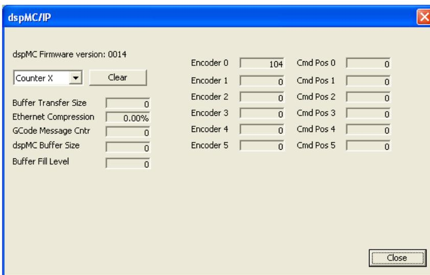
This screen is mostly used for diagnostics, but the user can also clear the Encoder counters, if required.
