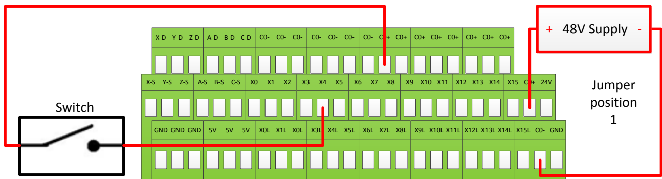
FIGURE 96 - HIGH VOLTAGE SOURCING INPUTS
