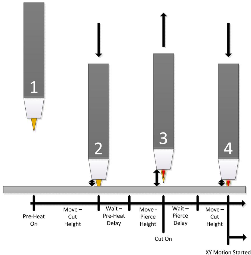
**Figure 8 - OxyFuel Cut Sequence**
