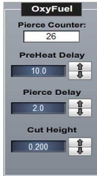
Figure 9 - Oxy Fuel Operating Settings
