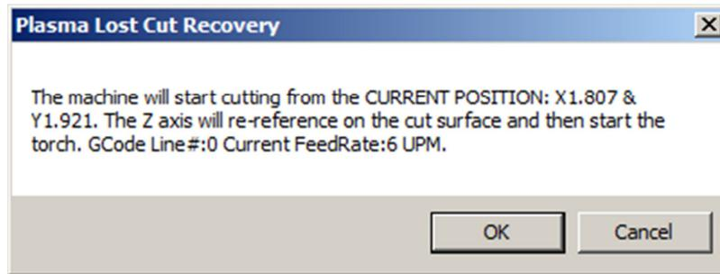
Figure 16 – Manual Plasma Lost Cut Recovery Dialog
