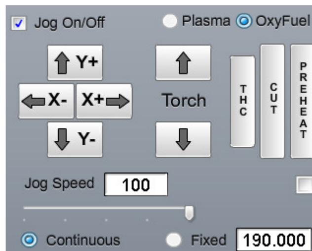
Figure 10 - Jog Controls on OxyFuel
