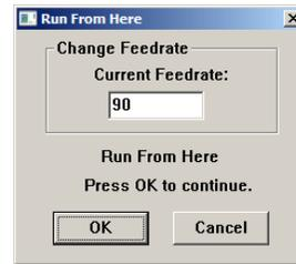
Your machine will move into position, re-reference the Z axis, and then begin cutting from the G-code line you selected.
