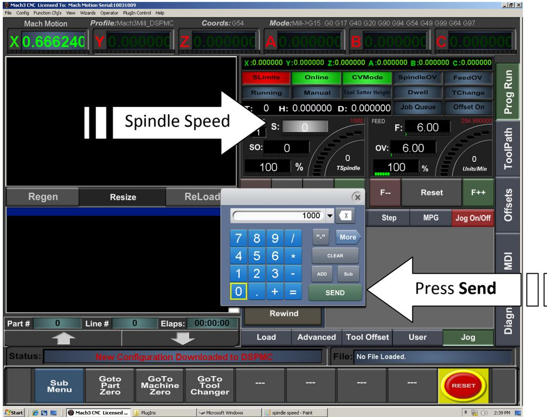
Figure 38 Setting up Spindle Speed
