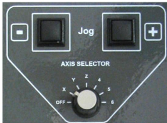
Figure 15 Jog Buttons and Axis Selector
