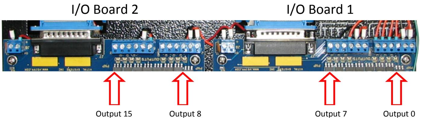
*Note: All outputs on the Interpreter are accessed in Mach3 with port 1 pin X where X is the output number.*
