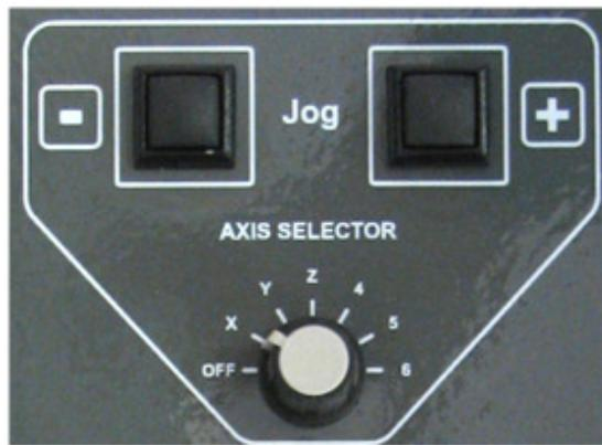
Figure 18 Jog Buttons and Axis Selector
