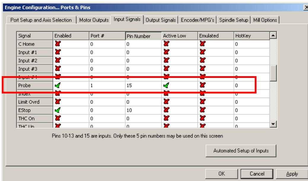
Figure 102 Probe Input
