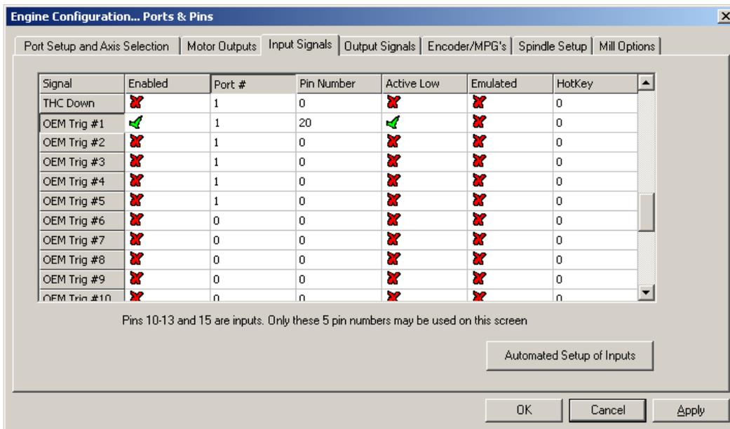
Figure 65 Example Input Configuration
