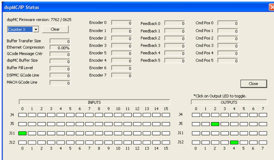
Figure 32 dspMC/IP Status Window
