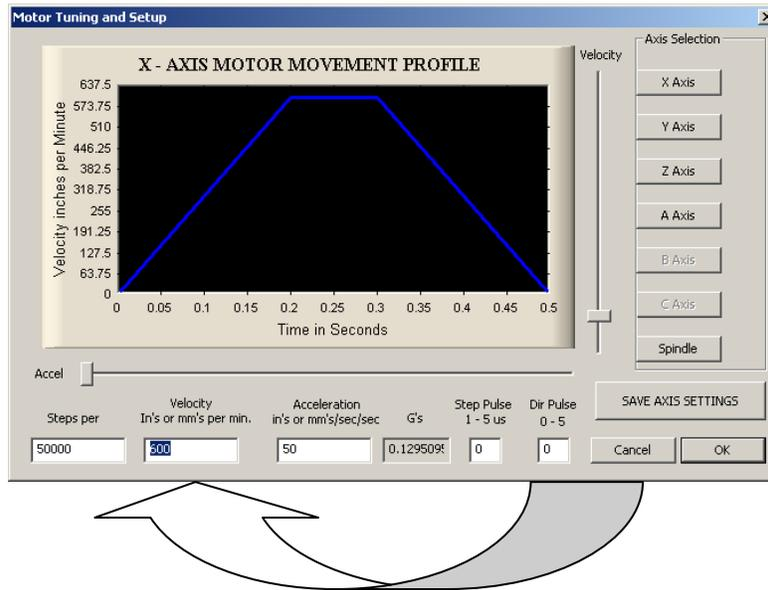
Figure 41 Velocity in Motor Tuning
