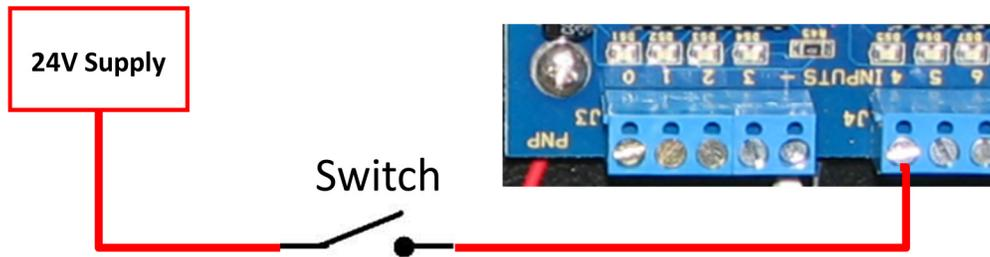
Figure 64 Example Input Wiring
