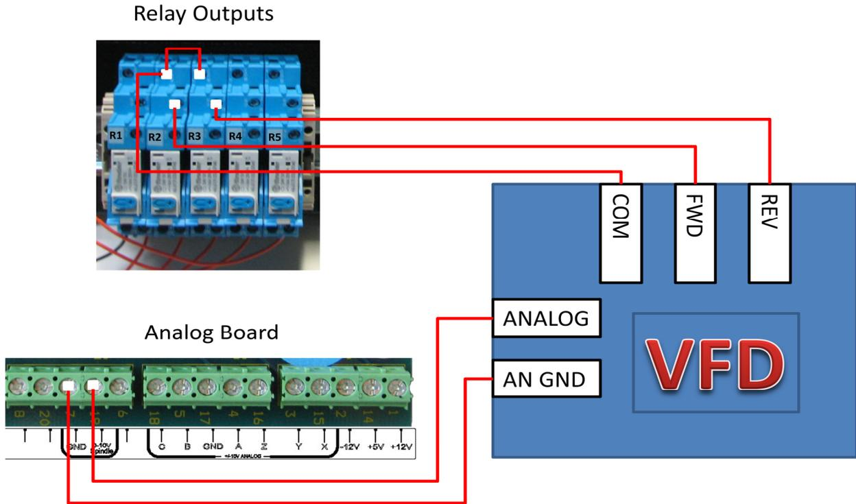
Figure 91 VFD Schematic
