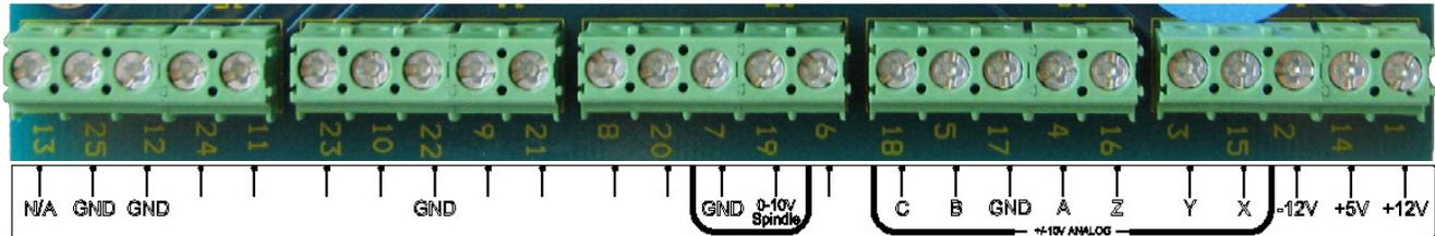
Again make sure to connect your shields to ground. Use the table below as a reference for your analog outputs.
