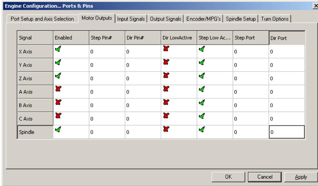
Figure 38 Axes Enabled
