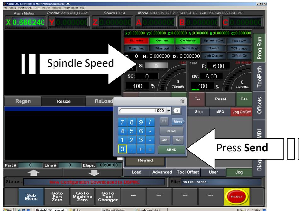
Figure 98 Setting up Spindle Speed
