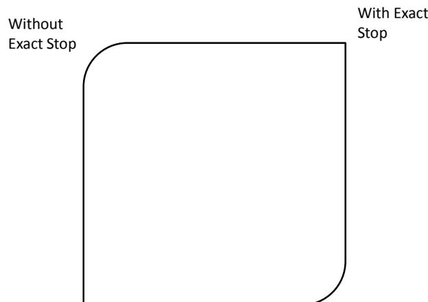
FIGURE 5 SQUARE WITH EXACT STOP ON TWO CORNERS
