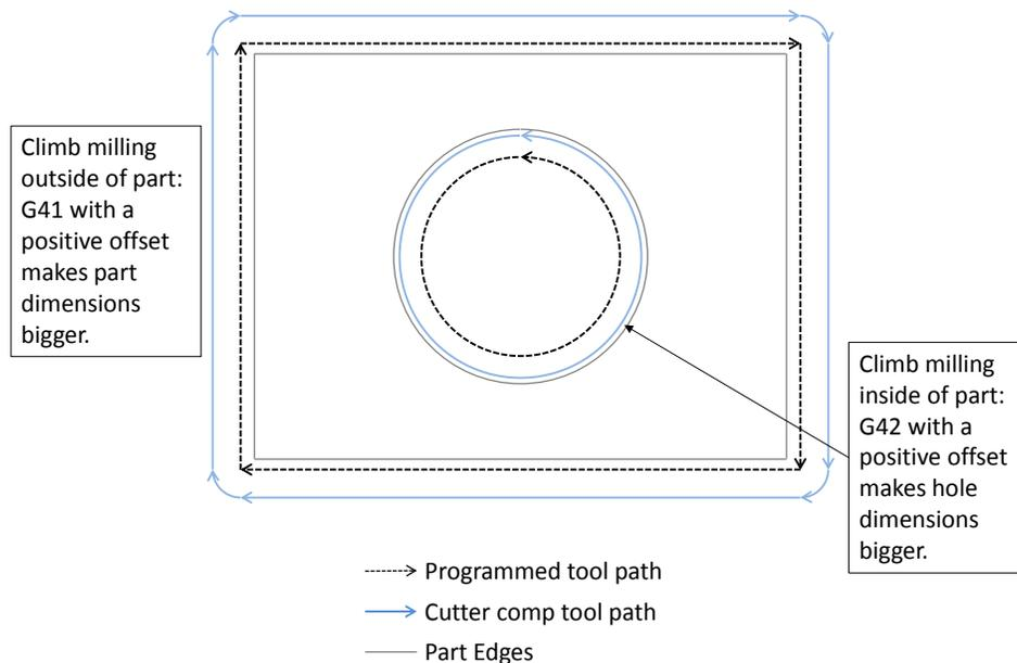
Figure 41-2: Cutter compensation OD and ID features.
