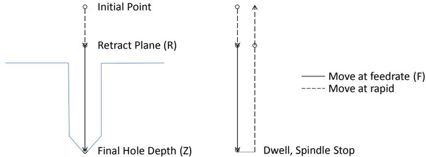
FIGURE 24 MOTION OF TOOL POINT FOR G86 CYCLE. END Z POSITION WILL BE DETERMINED BY G98/99 SETTING
