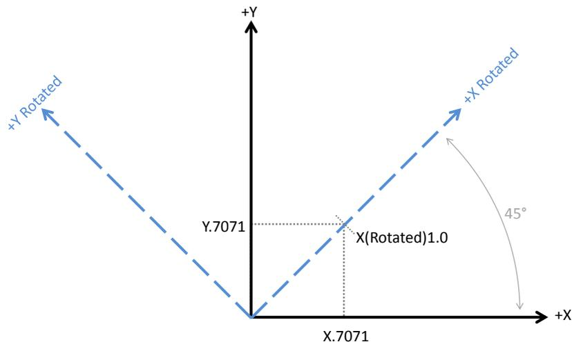
FIGURE 14 COORDINATE SYSTEM ROTATION (G68 X0 TO R45)
