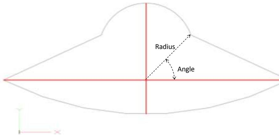
FIGURE 7 TOOL PATH OF POLAR COORDINATE MODE EXAMPLE
